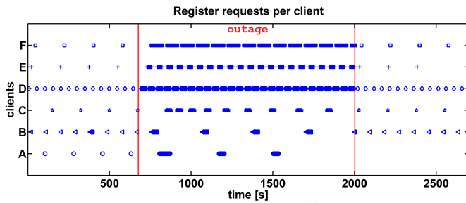
Fig. 7. Register requests of a few users demonstrating different registration patterns and client behaviour. Note that client A stopped trying and did not register again in the analysed trace. This per-user analysis is only possible thanks to the session-preserving feature of the SiAnTo anonymizer.
